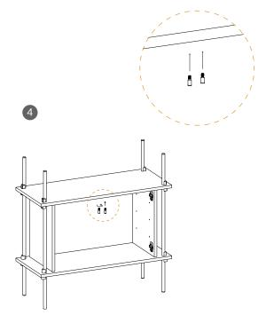
Insert the door stoppers by screwing them into the holes of the top shelf.
