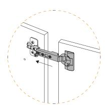
Slide the hinge over the metal plate.
