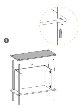
Slide down the top shelf until it sits on the dowels of the side panels. Fasten it with the wedges. Use a hammer to make sure it is secured.
