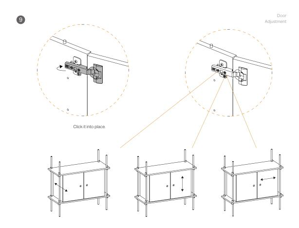
To adjust the placement of the doors, tighten/loosen these three screws.
