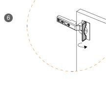
Place the hinges in the large holes of the doors.
