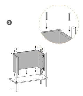
Insert the dowels into the holes of the back and side panels. Attach them to the bottom shelf.
