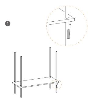
Start by placing the bottom shelf at a desired height, fasten it with the wedges. Use a water level and a hammer to make sure it is leveled and secured.
