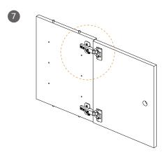
Mount the doors onto the side panels of the cabinet.
